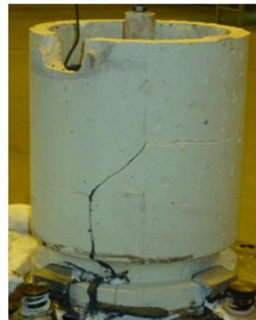
**Fig.18.** Crucible crack during the test.
